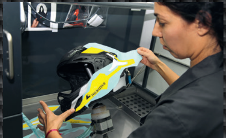
Decoration Decoration is applied to the finished helmet. A steady hand is needed to piece together the individual foils.
