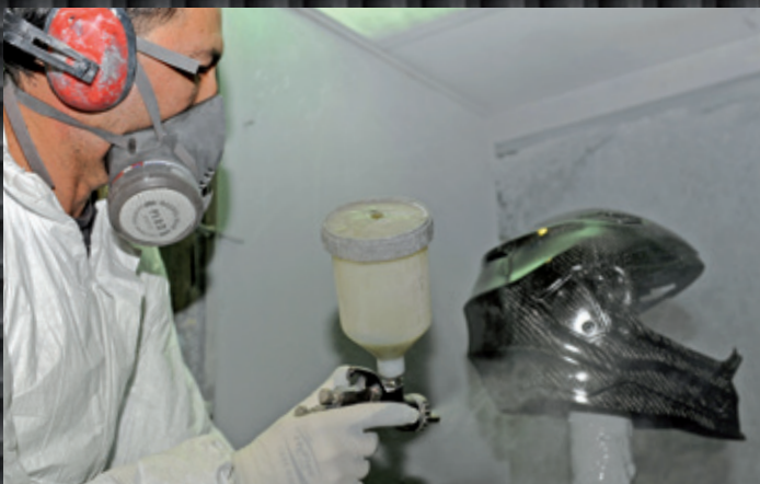
Smoothing and coating Fillers and protective lacquers are applied in several stages. The helmet is re-polished between each step.
