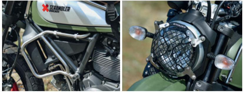
The robust guard made from electropolished stainless steel protects the radiator (l). Headlamp grill provides stylish protection.
