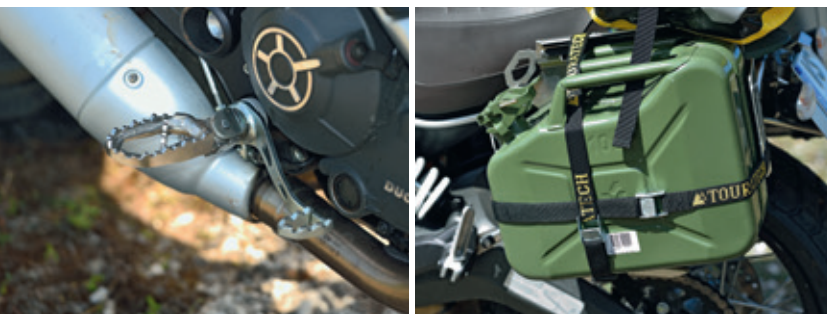
Broad, serrated foot pegs provide stability off-road (l). Robust – metal canister on a sturdy stainless steel holder.
