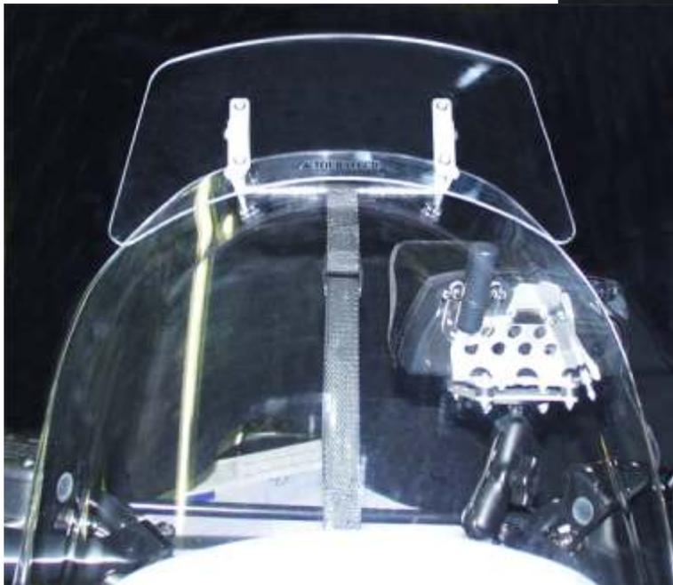
Push the spoiler with the two guide slots into position at the center of the windscreen. You may need to apply some force to the spoiler so that it seats firmly in place at the top of the screen. Take care that the slots bottom out otherwise you run the risk of scratching the screen. The hook of the strap grabs underneath the plastic shroud between the screen and the instrument panel.
