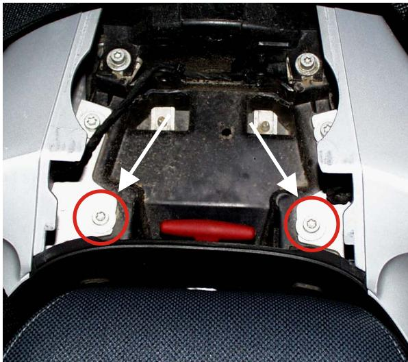
Exchange the two marked screws on the inside of the luggage compartment for the two enclosed screw caphead M6x35 with one large M6 washer each. You must fully tighten these two screws before further mounting, since the screws fit in threaded mounts in the subframe and cannot be pulled tight later. The screws should now come through the bottom surface far enough to mount the license plate reinforcement.
