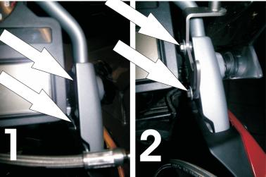
2nd OPTION) Remove headlight guard if such is installed. Loosen the bolt on both side that supports the complete headlight/instrument panel unit. This bolt is right between the blinker and the windshield adjustment.
