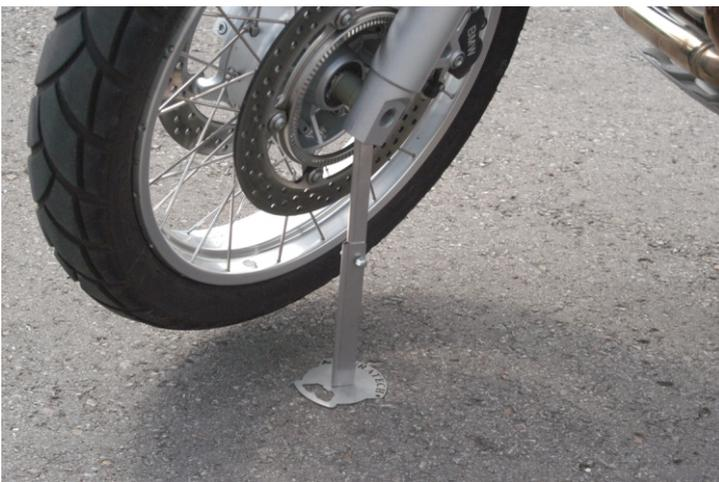
Turn the front wheel to the left and lock the steering lock with your ignition key. Attach the top and lower wheel removal jack parts together with the supplied screw and nut. Put the sharper point of the wheel jack into the hole on the left front fork and the lower part on the two small holes on the ground plate.
