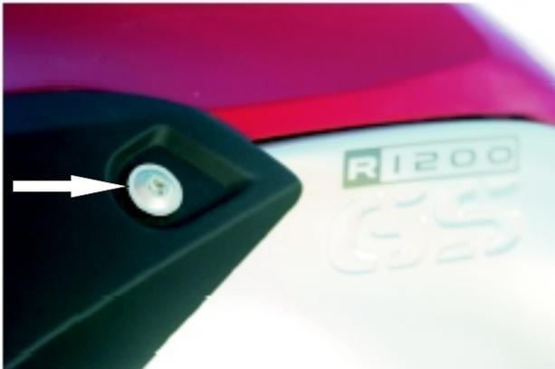
Nice looking fasteners to replace the stock ones. Touratech Phillips head side cover fasteners prevent from unwanted side cover removal better than stock ones.
