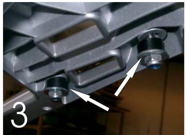
Make sure all spacers are correctly positioned and recheck the tightness before your ride and periodically
