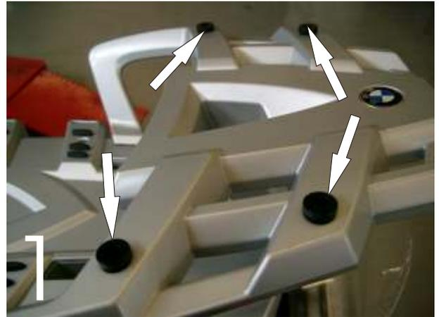
Set the rack extension on the spacers and put the screws through from the top as shown on photo 2.
