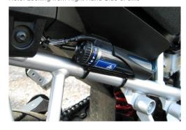
The Dispenser Assembly can be secured to the paddock stand bobbin mount using the small Dispenser Plate & Clip, parts 20 & 21. The delivery tubing can be routed along the swing arm using self adhesive cable clips. For further information see our easy step installation guide - <u>Dispenser Assemblies</u>, <u>General</u>. The nib should feed the rear sprocket between the 6 & 7 o'clock positions, with the cut face facing outwards.
